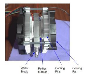
Figure 3, the assembled Peltier Cooler
