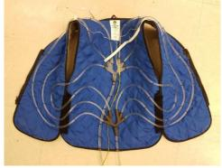
Figure 4, Tubes and water junctions sewn onto inside surface of the vest.
