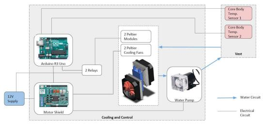
Figure 2, Schematic of electrical (black lines) and fluid (blue lines) circuits
