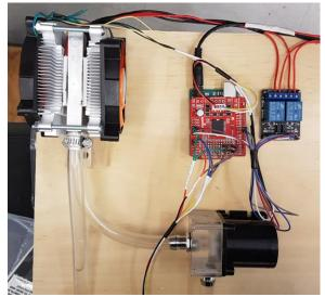
Figure 5, (top) the completed prototype with the vest turned inside out; (bottom) close-up of the cooling and control board showing cooler, pump, Arduino controller and relays.
